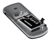
To insert the battery, insert the battery into the opening on the back of the phone at an angle (1), making sure the metal contacts on the battery connect with the matching connectors in the phone. Press down until the battery snaps into place (2).
