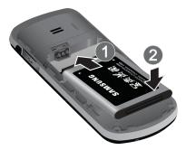
4. Replace the cover plate by lining up the tabs and then firmly sliding the cover in the direction of the arrow (2) until it snaps into place.
