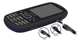
Note: The previous illustration displays the incorrect method for connecting the charger. If attempted, damage to the accessory port will occur therefore voiding the phone's warranty.
